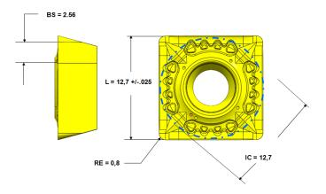
Figure 34: Indexable Insert Measurements
