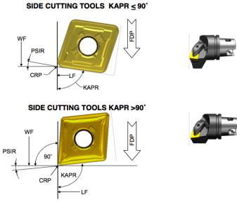
Figure 30: Cutting Tool Measurement Diagram 4 (Cutting Item – ISO 13399)
