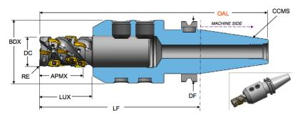
Figure 18: Cutting Tool Measurement Diagram 1
