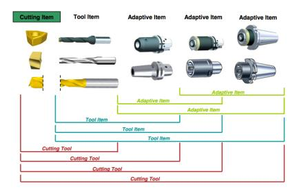
Figure 3: Cutting Tool Composition
