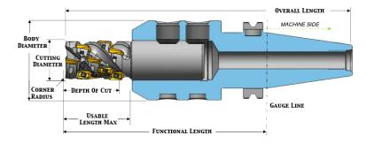
Figure 6: Cutting Tool Measurements
