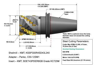
Figure 33: Shell Mill Side View
