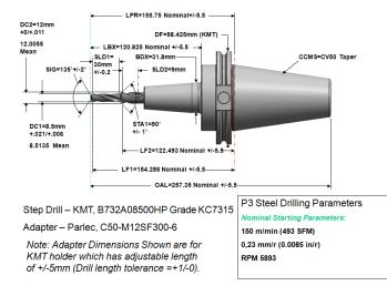
Figure 35: Step Mill Side View
