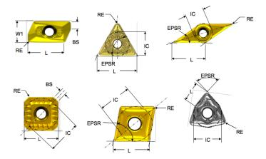
Figure 29: Cutting Tool Measurement Diagram 3 (Cutting Item – ISO 13399)
