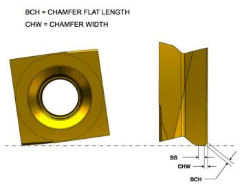
Figure 32: Cutting Tool Measurement Diagram 6 (Cutting Item – ISO 13399)
