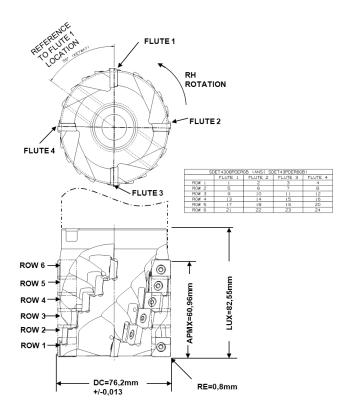
Figure 36: Shell Mill with Explicate Loci
