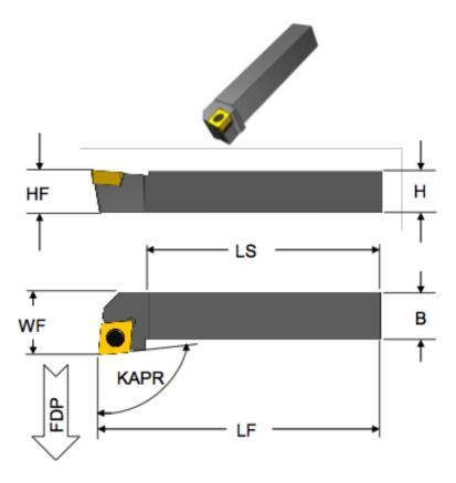
Figure 19: Cutting Tool Measurement Diagram 2
