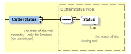
Figure 9: CutterStatus Schema
