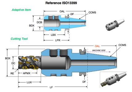
Figure 5: Cutting Tool, Tool Item, and Cutting Item 2
