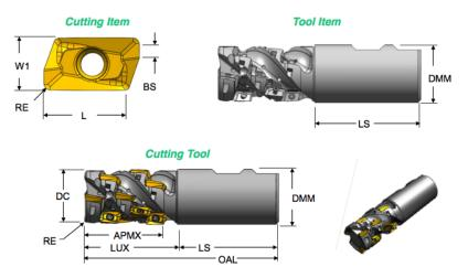
Figure 4: Cutting Tool, Tool Item, and Cutting Item
