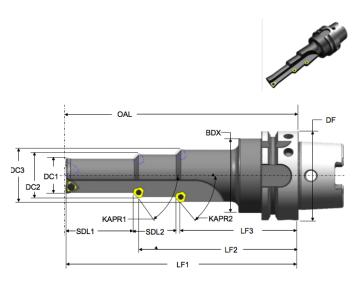
**Figure 27:** Cutting Tool Measurement Diagram 1 (Cutting Tool, Cutting Item, and Assembly Item – ISO 13399)
