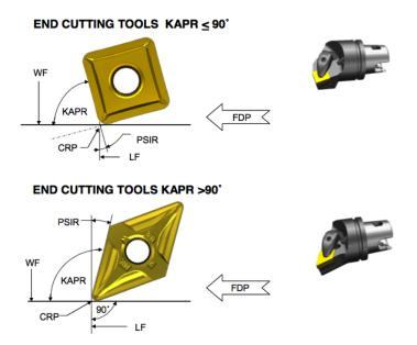
Figure 31: Cutting Tool Measurement Diagram 5 (Cutting Item – ISO 13399)
