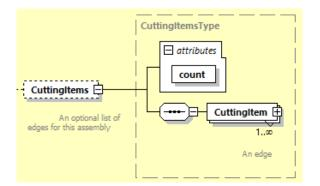
Figure 20: CuttingItems Schema
