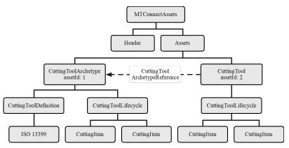
Figure 7: Cutting Tool Asset Structure
