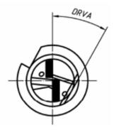
Figure 26: Cutting Item Drive Angle
