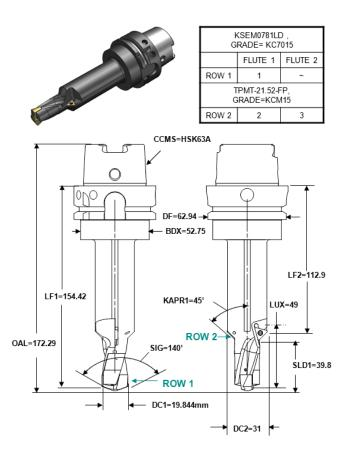
Figure 37: Step Drill with Explicate Loci
