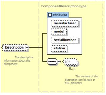
Figure 7: Schema for Description of Component
