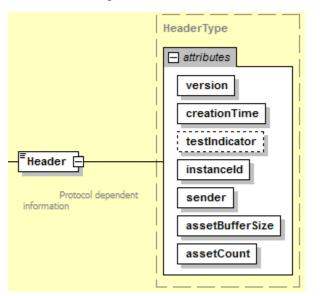
Figure 12: Header Schema Diagram for MTConnectAssets
