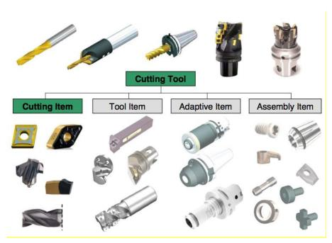
**Figure 2: Cutting Tool Parts**
